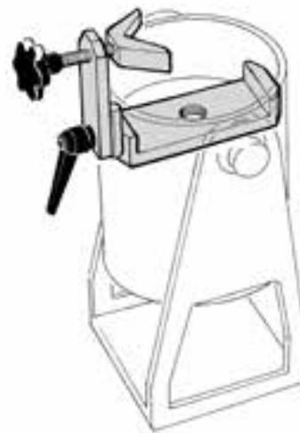
Clamping device for threaded bits (87002401) in Manual B-DTH grinding machine.
