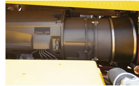
Standard imported Deutz 4-cylinder, TCD3.6 L4, 55.4 kW, Chinese Stage III, environmental friendly.
