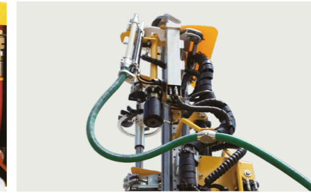
Hose injection system for resin cartridges, shooting the cartridges from the operator's platform, injecting through a foldable nozzle in front of the feed.
